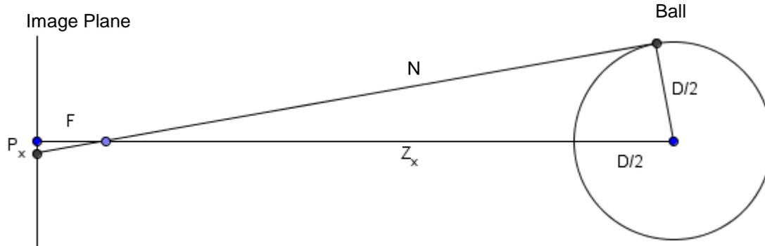
Figure 2. Simple Diagram for Frame  $x$  (side view)
